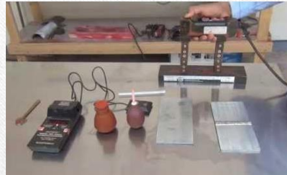
Magnetic Particle Testing (MT)
