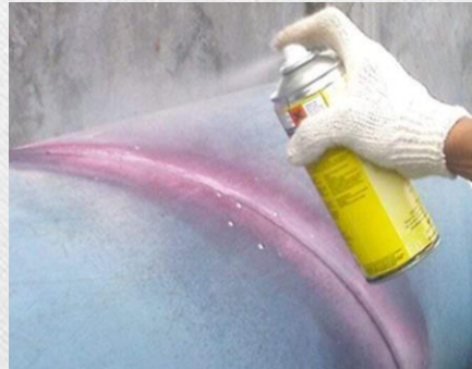
Dye Penetrant Test (DPT)
